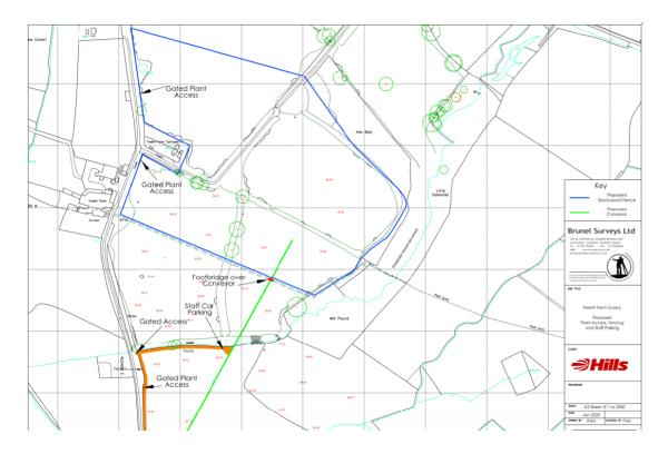
28. To erect and dismantle the conveyor bridge, a crane will be required to operate from within the agricultural field in which the conveyor is located. It is therefore proposed to
