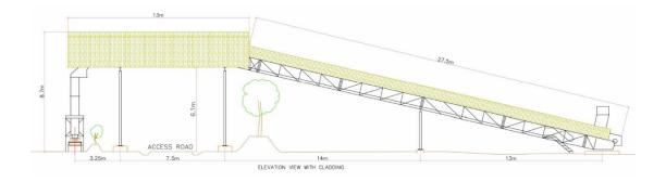
23. The foundation slabs and upright sections of the conveyor bridge can be erected without disturbance to the users of the lane leading to Freeth Farm. The horizontal section of the crossing will be erected using a crane, located in the adjacent field. As this point, the use of the road will need to be restricted for approximately 2 hours. The
